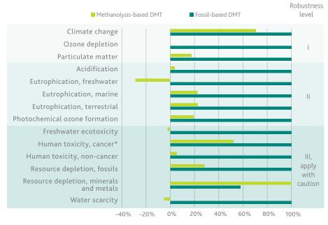
**Goal of study**: Complete LCA of recycled dimethyl terephthalate (DMT) produced by methanolysis from polyester waste and compare to conventional DMT produced by Eastman at the same site from fossil-based paraxylene.
